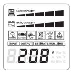
The multifunction LCD readout provides ready access to power/battery condition vitals, such as: Runtime, Load, Temperature, and much more. The screen is also rotatable so the UPS can be used in either rack mount or vertical/tower orientation.
